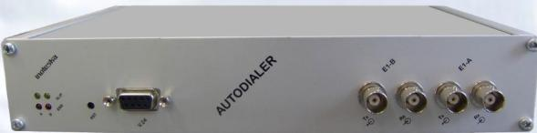
Least-cost voice router for PRI/E1 interface. Router is being installed between PBX (Private Branch Exchange) and Public Exchange.
